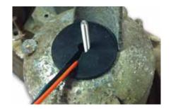
Use the end of the screw to adjust the LED panel into its final position. Place the slotted washer on top of the grommet. Then slide on the nylon washer and screw it all together with the black wing nut. Tighten snug until the LED panel is fit snug in place. Make sure that the LED panel is not bending in from too much tightening force. You may want to use loctite or silicone to make sure the wing nut stays secure. DO NOT OVER TIGHTEN WING NUT.
