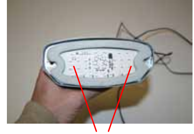
LED panel sits into mounting screw.
