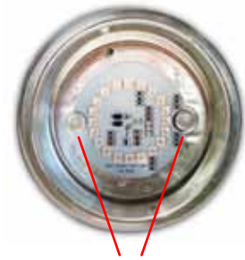
LED panel sits into mounting screw.
