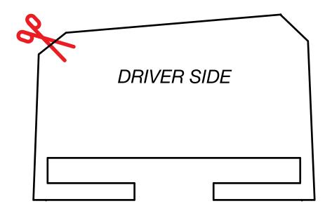
Cut out the templates and position them on the bottom side of the taillight housing.
